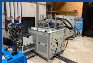
120 kW PEM fuel cell test bench dedicated to industrial projects
