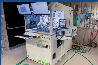
PEM electrolyzer test bench 1 kW
